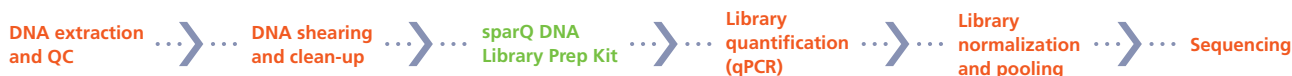
Figure 1 Overview of the workflow for preparation of NGS libraries using the sparQ DNA Library Prep Kit.
