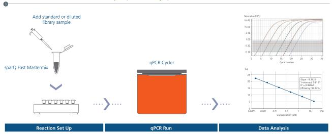
Illustration of sparQ Fast Library Quant Kit workflow. Reactions are prepared by simply adding standard or diluted library sample. Optimized protocols with fast cycling condition are provided for both 10 µl or 20 µl reaction volumes.
