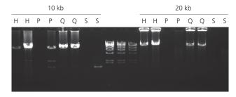
4.14 Long Range capabilities ( $\lambda$ DNA). A range of 10 kb, 20 kb, 30 kb, and 40 kb  $\lambda$ DNA templates were amplified with varying GC-content and lengths using each manufacturers recommended cycling conditions. The experiment was run in duplicate.
