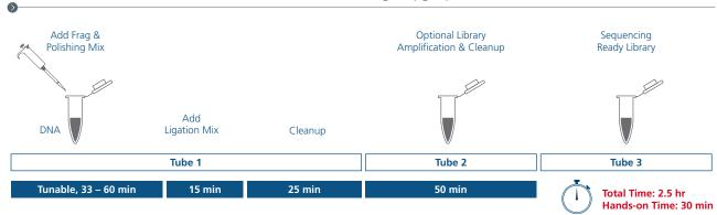
The streamlined workflow utilizes a proprietary enzyme mix that combines fragmentation and DNA polishing in a single step to simplify library construction. High efficiency adapter ligation and cleanup are performed in the same tube, followed by an optional amplification step using HiFi PCR Master Mix and Primer Mix.
