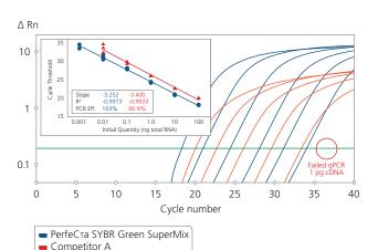
420 PKCA target amplified from log-fold serial dilutions of qScript synthesized cDNA from HeLa cell total RNA (100 ng – 1 pg) with either PerfeCτa SYBR Green SuperMix or Power SYBR Green PCR Master Mix.
