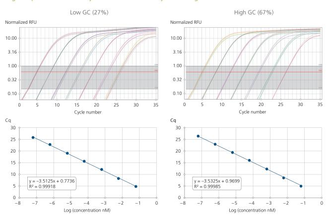
sparQ Fast Library Quant Kit provides high amplification efficiency across a wide linear dynamic range. A 10-fold dilution series was prepared from libraries of low (27%) and high (67%) GC-content and amplified under fast conditions on the Q using the sparQ Fast Mastermix. The slopes of the Cq vs Log (concentration) plots and the individual sample reactions measured by the LinRegPCR algorithm indicated superb amplification efficiencies.
