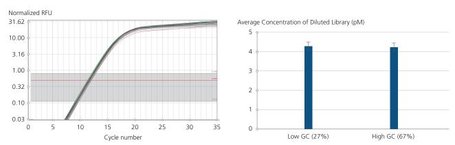
Multiple runs using sparQ Fast Library Quant Kit resulted in similar quantification values. Two NGS library preparations with high and low GC-contents were amplified and quantified in five distinct runs. Plots of the Normalized fluorescence vs Cycles and average quantification values show the high repeatability of measurements with the sparQ Fast Library Quant Kit under fast cycling on the Q.
