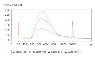
amplification from low input. The fragment size distribution and the quality of the amplified DNA libraries from 250 pg input DNA were analyzed using a high sensitivity DNA analysis kit on the Agilent BioAnalyzer. Libraries were amplified using sparQ HiFi PCR Master Mix (orange) or equivalent kit from Supplier K (blue) and Supplier N (red) with identical amplification cycle numbers (16 cycles for 250 pg input DNA).
