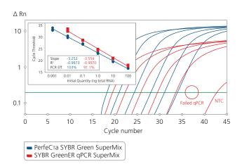
PKCA target amplified from log-fold serial dilutions of qScript synthesized cDNA from HeLa cell total RNA (100 ng − 1 pg) with either PerFeCTa SYBR Green SuperMix or SYBR GreenER™ qPCR SuperMix.
