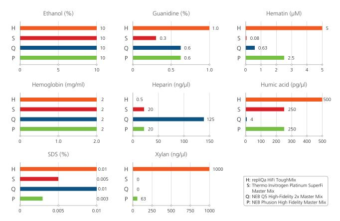
Strong Inhibitor Resistance. A 2 kb  $\lambda$  DNA template was amplified using each manufacturers recommended cycling conditions with different amounts of inhibitors. The experiment was run in duplicate.
