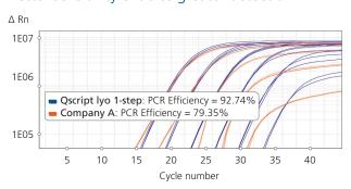
Qscript lyo 1-step demonstrates higher sensitivity and fluorescence signal than a market-leading one-step RT-qPCR product (liquid). The figure shows a LDHA assay with 10-fold serial diluted universal human RNA (50 ng to 0.5 pg) as template. 20 µl of LDHA primer/probe was used to resuspend each lyosphere, followed by addition of 5 µl of RNA target. RT-qPCR was carried out on a QuantStudio 7 instrument with the following conditions: 50°C 15 min, 95°C 3 min, 40 cycles: 95°C 15 sec, 60°C 60 sec.
