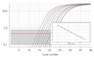
4.3 Manganese superoxide dismutase gene (MnSOD). Eight point, 2x dilution series of human genomic DNA (n = 4 each); Efficiency = 98% (standard curve method); R<sup>2</sup> = 1.00
