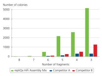
PCR fragments containing 30 bp overlaps were Dpnl treated, purified, and assembled according to the protocol. Reactions contained the indicated number of DNA fragments (0.1 pmol each) and were incubated at 50 °C for 60 minutes. 1  $\mu$ l of the reactions were used to transform 30  $\mu$ l of chemically competent cells.
