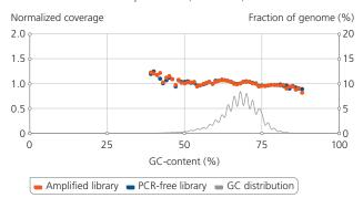
Consistent coverage over a broad range of GC-content with sparQ HiFi PCR Master Mix. Libraries were prepared by using sparQ DNA Library Prep Kit with 100 ng input DNA. Coverage depth against GC-content of libraries amplified by sparQ HiFi PCR Master Mix (red) were compared to corresponding libraries without amplification (dark blue: PCR-free library). GC-content distribution of targeted genomes is indicated by the gray line.
