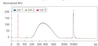
Highly reproducible DNA library profiles were achieved using different lots of sparQ PureMag Beads and a broad range of input amount. Libraries were prepared with sparQ DNA Library Prep Kit from 100 ng and 1 ng of fragmented microbial genomic DNA. sparQ PureMag Beads were used post adapter ligation and PCR amplification to effectively remove adapter-dimers and primer-dimers.
