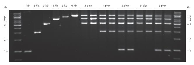
5 trong multiplexing capabilities. Multiplex PCR reactions were performed for amplification of 2 kb, 3 kb, 4 kb and 5 kb BRCA 1 targets with 1 kb and 6 kb BRCA 2 targets from 10 ng human genomic DNA template. Reactions were run on MJ Research PTC-200 Thermal Cycler. Following a 2 min activation of 95°C; 27 cycles of PCR were performed: 92°C, 30 s, 65°C, 8 min; 72°C, 10 min. 4 µl of PCR products were analyzed on a 0.7% agarose gel.
