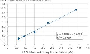
Results from sparQ and Roche KAPA Library Quant Kits were highly correlated. Concentrations of six different diluted libraries were determined using either the sparQ Fast Library Quant Kit on Q or the Roche KAPA Library Quantification Kit on Bio-Rad CFX following the manufacturer's recommended protocol. Run times, including melt curves, were 40 minutes for sparQ and 80 minutes for KAPA.
