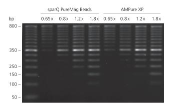
sparQ PureMag Beads show equivalent performance to AMPure XP for DNA purification. 50 bp DNA ladder was purified with sparQ PureMag Beads and AMPure XP at different beads to DNA ratios and analyzed on 2% agarose gel.
