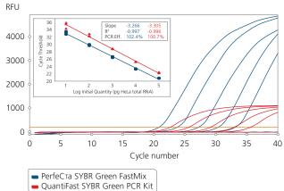
ADAR target amplified from log-fold serial dilutions of qScript synthesized cDNA from HeLa cell total RNA (100 ng – 10 pg) with either PerfeCTa SYBR Green FastMix or QuantiFast SYBR Green PCR Kit.
