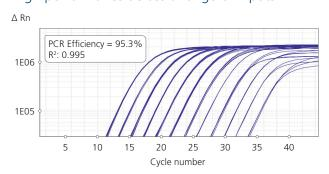
3.8 Qscript lyo 1-step was tested with 12 serial dilutions of Human total RNA (4x from 1250 ng to 0.3 pg). 20 µl of LDHA primer/probe was used to resuspend each lyosphere, followed by addition of 5 µl of RNA target. RT-qPCR was carried out on a QuantStudio 7 instrument with the following conditions: 50°C 15 min, 95°C 3 min, 40 cycles: 95°C 15 sec, 60°C 60 sec.
