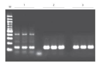
4.19 Amplification of a 131 bp TNF fragment using different 5PRIME Taq enzymes.
