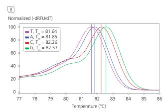
555 Effect of T,A,C, or G variant base on T<sub>m</sub> in a model HRM SNP system with either AccuMelt HRM SuperMix (Panel A), or a competitor's SYTO 9 dye master mix (Panel B). Plots of averaged melt peaks normalized to maximum signal for each system.
