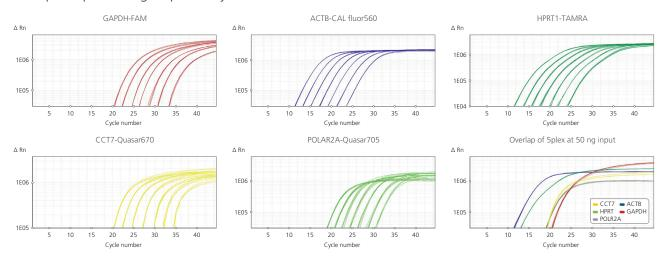
232 Qscript lyo 1-step was tested with a 5-plex assay with 7 serial dilutions of Human total RNA (4x from 50 ng to 30 pg). 20 µl of primers/probes was used to resuspend each lyosphere, followed by addition of 5 µl of RNA target. RT-qPCR was carried out on a QuantStudio 7 instrument with the following conditions: 50°C 15 min, 95°C 3 min, 40 cycles: 95°C 15 sec, 60°C 60 sec.
